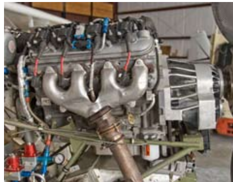
What do you get when you cross a small-block V8 Chevy engine with a standard, run-of-the-mill 172? The Chevssna.
